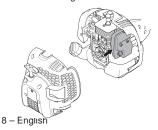
In countries that have a warm and dry climate there is a significant risk of fire. We therefore fit certain mufflers with a spark arrestor mesh. Check whether the muffler on your machine is fitted with this kind of mesh.
