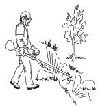
Keep a good balance and a firm foothold. Do not overreach. Keep proper footing and balance at all times.
