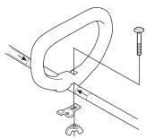
Fit the bolt, securing plate and wing nut as shown in the diagram. Tighten the wing nut.
